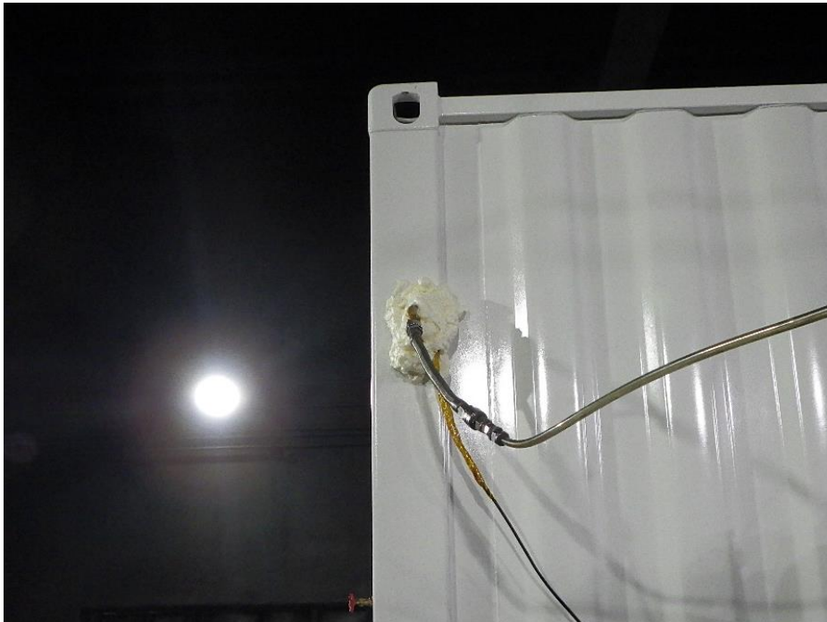
Figure F4 – Photo of the hoses going through the container wall and the urethane seal
