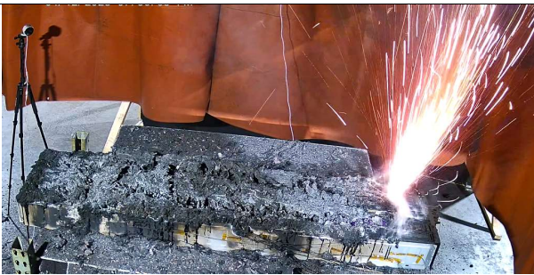
(k) Continued Thermal Runaway 04:35:51
