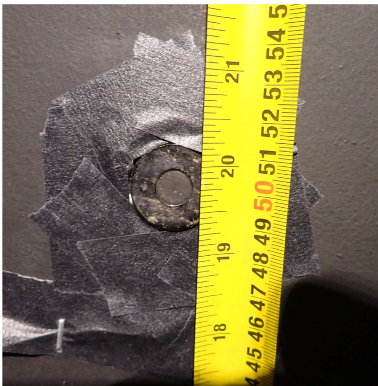
Figure C10 - Heat Flux Installed in the Side Wall at Initiating Module Height
